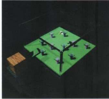
Fig. 1. Schematic representation of the basic setup used for laboratory colour preference experiments. The wooden nestbox (left), containing the bumblebee colony, is connected to a flight arena (right) via a clear Plexiglas tube. The experimenter can control the traffic of bees passing from the nest into the arena (and vice versa) using shutters along the length of the connecting tube. The flight arena contains one or more types of artificial flowers, which differ in colour and presence of reward depending on precise training and test conditions (see methods for full details). Figure design courtesy of R. Beau Lotto.
